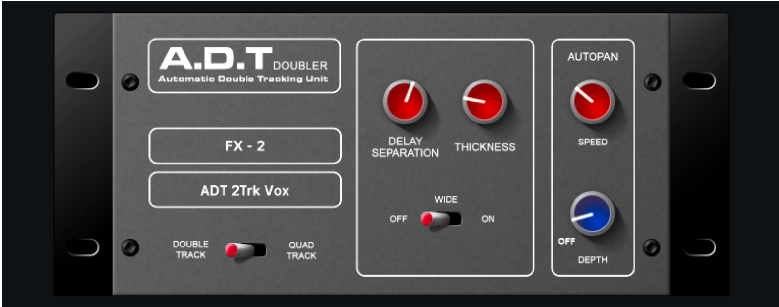
Automatic double tracking unit with Double Track and Quad Track modes along with Separation , Thickness and Autopan .
