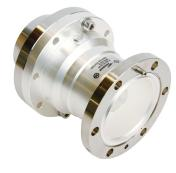
3-1/8 in EIA Female Flange with gas barrier for 3 in HJ8-50B air dielectric cable. Coupling Element, O-Ring, screw-set sold separately. Click-on: Related Products, Device connectors and Adapters
