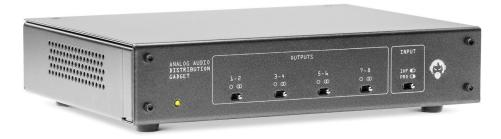
On the input side, the Distribution Gadget offers a choice of unbalanced IHF RCA inputs featuring our exclusive "ground (loop) breaking" circuity or high CMRR balanced pro inputs on XLR connectors. A front panel switch allows input switching on the fly.
