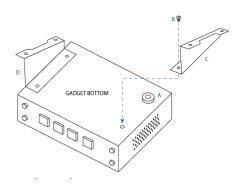
Use the four provided No. 6 screws ("E") and cup washers ("F") as shown in the diagram above to secure the gadget to a plywood surface.
