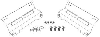
Remove the four rubber feet ("A") from the bottom of the gadget using a #1 Phillips screwdriver, being careful to save the screws.
