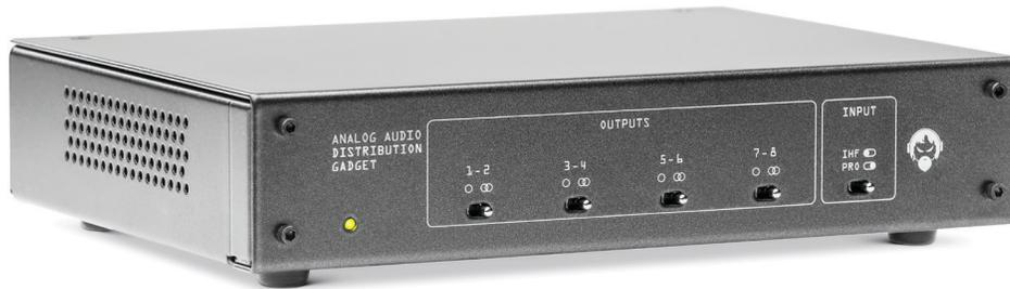
The Distribution Gadget allows a single source to drive multiple destinations. This is especially useful in broadcasting for connecting the studio output to an air chain, internet encoder, recording device, etc. The Distribution Gadget eliminates the ground loops and signal loss that often occur when directly attaching multiple loads to a source.
