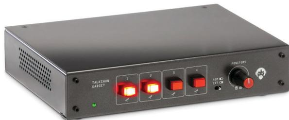
Enter the Talkshow Gadget, which allows you to add these useful broadcast features to your live mixer. It features instant muting switches for four microphone inserts, a level control for your monitor speakers, an input for monitoring an external source, and dry relay contact closures which follow the status of the microphones. Each microphone has its own mute override logic signal should you not wish to mute the monitor output.
