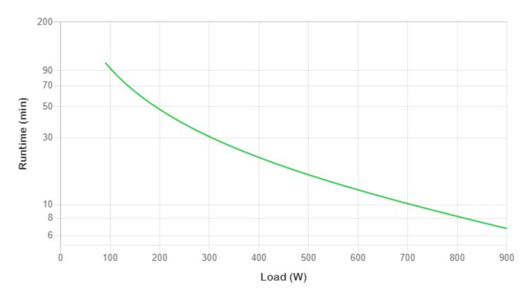
Curve fit to measured runtime data. All measurements taken with new, fully charged batteries, at typical environmental conditions, with no electrical input and balanced resistive load (PF = 1.0) output.
