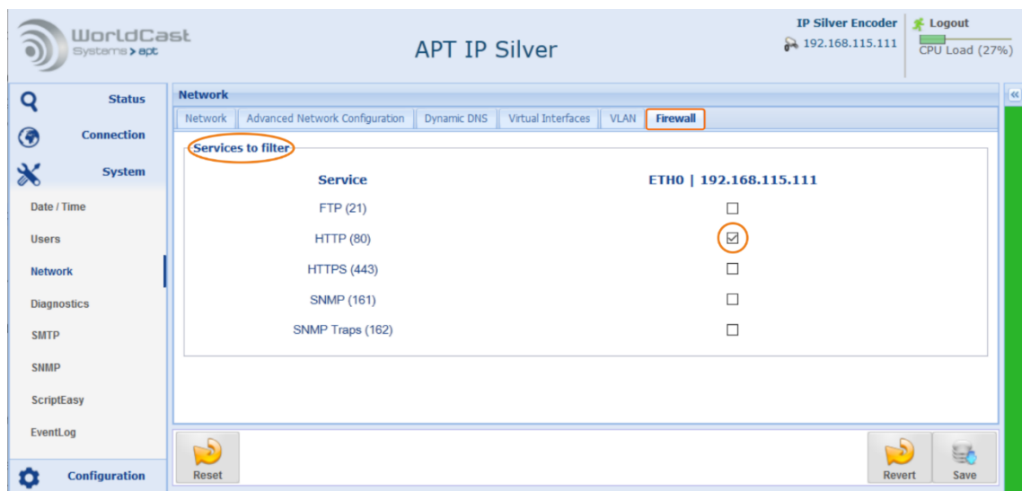
Figure 3-50: Shows the filter options on the firewall page - HTTP service (port 80) is disabled on both interfaces
