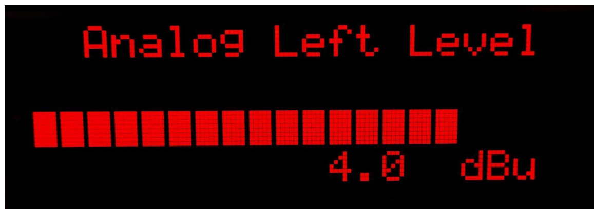
Figure 3.2.15: Output Mono Left Level Control Screen
