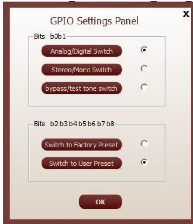
Figure 6.2: GPIO Settings Panel
