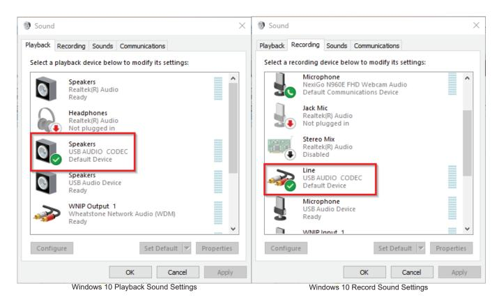
Above graphics show how the console will appear in the "old school" Windows Control Panel. The Windows Control Panel is reportedly being deprecated by Microsoft. If you no longer have Control Panel, you will need to go to **Settings | Sound** in Windows to find the AML's USB devices. The new settings windows are shown below:
