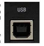
The USB input channel features a machine start logic signal. If you are running music playout software or an application such as Wheatstone's Voxpro editing system, you can start playback remotely from the console's
