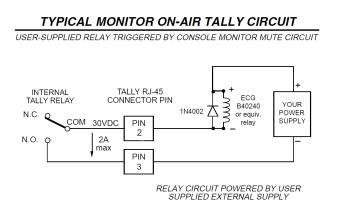
All machine start outputs are open collector and are active low. The tally signal is an optoisolated set of "contacts" that can be used to drive a user-supplied low-voltage relay to control Getting to Know the DML LYRIC
