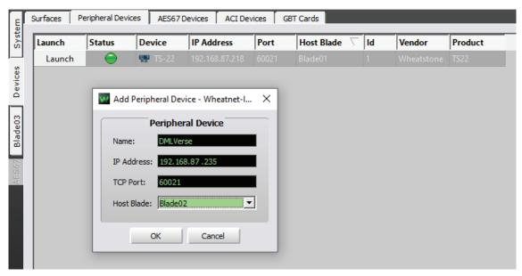
The default IP address of the DML LYRIC is 192.168.87.235. See the Blade-3 or Blade-4 manual for information on adding a device to the Peripheral Devices tab. When enabled, all three PGM busses are capable of simultaneously streaming from the DML LYRIC into the WNIP network.
