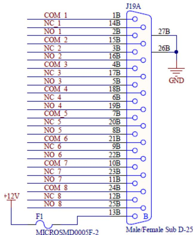
**i** Ground for the 12 V power supply is available on the ground of the unit.
