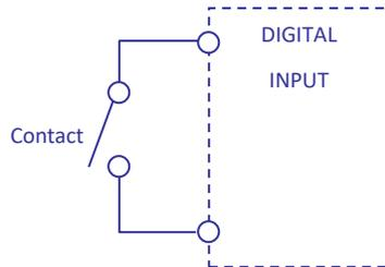
When a digital input is connected with the common, this input's value switches to '1'; otherwise it stays on '0'.
