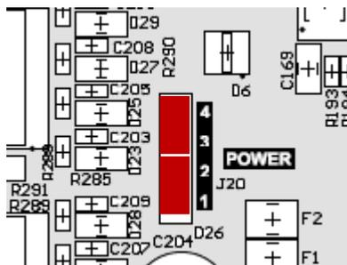
In internal power supply mode, 2 jumpers are on 1-2 and 3-4.
