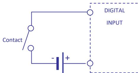
An external power supply between 5 and 25 V is applied to the common. If a digital input is connected to the ground, this input's value switches to '1'; otherwise it stays on '0'.
