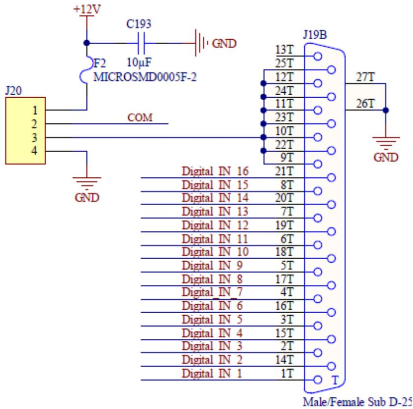
**i** When the 'internal power supply' mode is selected, the common ground is also the unit's ground.
