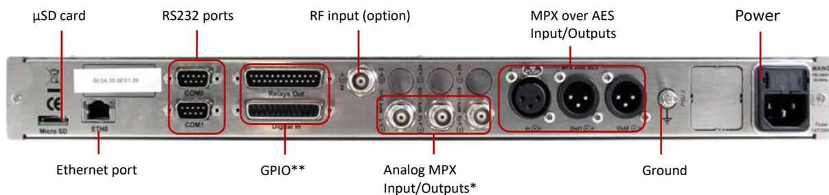
\* When the Audemat RDS Encoder is off, a signal on the input will go directly to the A output. There will be no signal on the B output.
