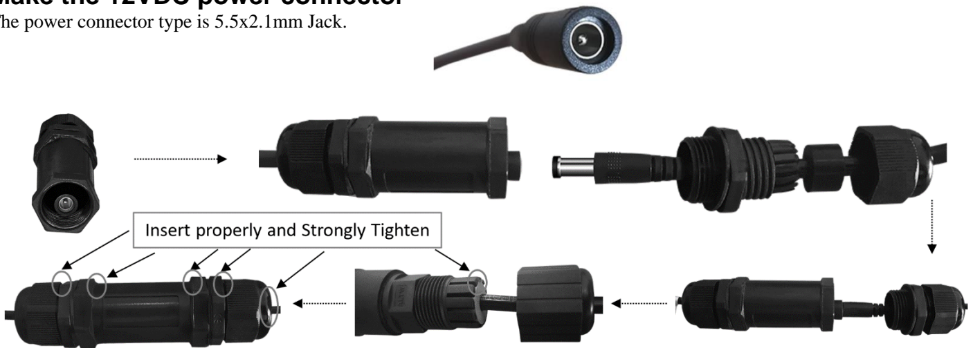
12VDC Power Connector + Waterproof Coupler Installation
