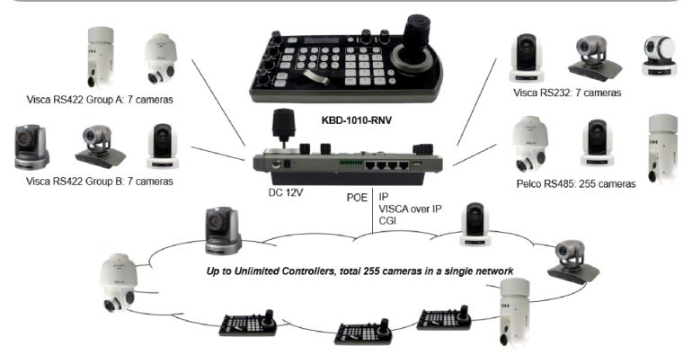
Cross Protocol Mix-control with RS232/RS422 and IP in one single system.
