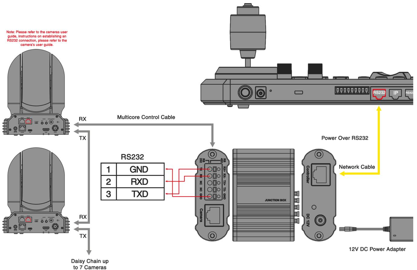
5. RS232 Connection: Using an RJ45 to Phoenix Connector Adapter (Sold Separately).
