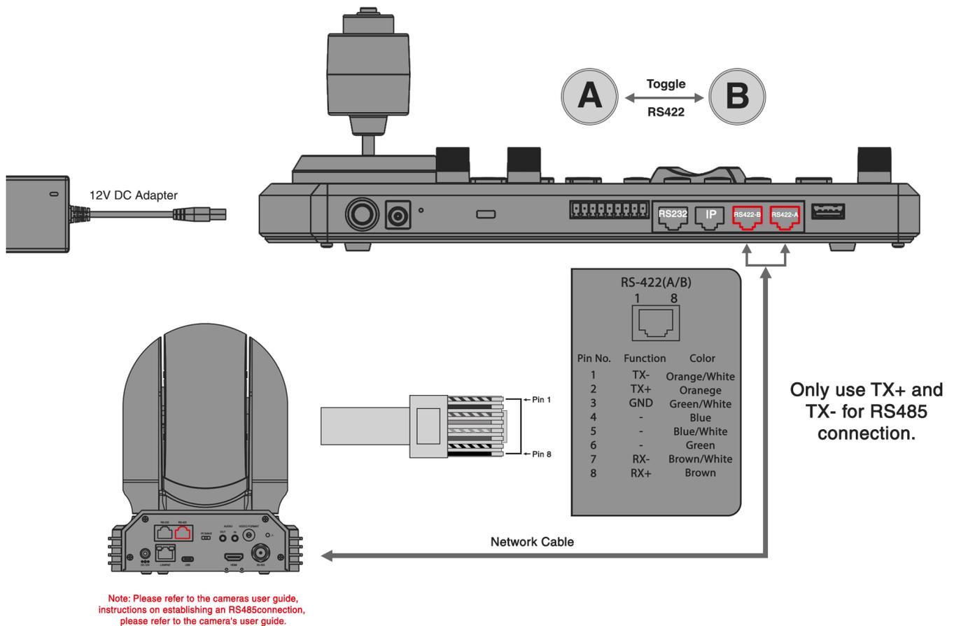
b. Follow the pinout for the RS485 port on both the keyboard and the Junction Box. Use a CAT5/6 cable, ensuring it adheres to the T-568B standard pinout between the keyboard and the Junction Box, to create a suitable cable for controlling your camera via the Junction Box.
