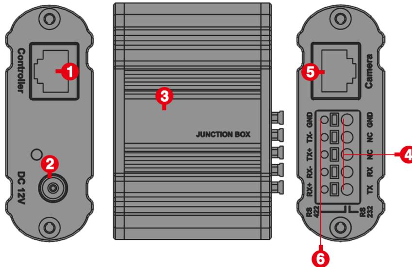
1. **RJ45 port** - connection between Junction Box and The Keyboard Controller.
