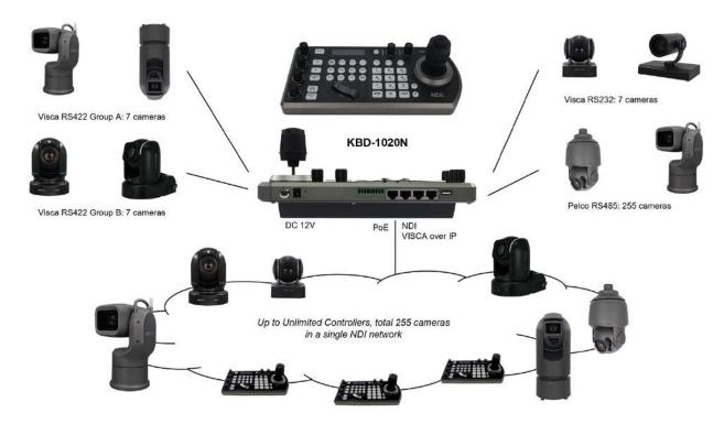
Cross Protocol Mix-control with IP and Serial RS232/RS422 in one single system.
