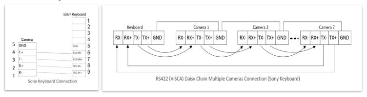
10. How to make RS422 connection and RS422 Daisy Chain multiple cameras connection with Non-Sony controller as below:
