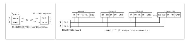
Use extension cables included RJ45 to RS422 Phoenix connecter adaptor to make RS485 connection for your control device.
