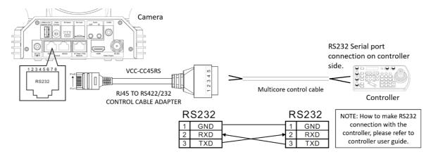
11. Or you can use CAT5/6 network cable **(T-568B standard pinout)** to make RS232 connection by following the pin definition below:
