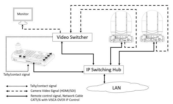
Tally Light GPI Connection – Using VISCA OVER IP Control Protocol
