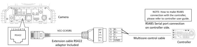
• Or you can use CAT5/6 T-568B Standard Ethernet cable direct connect between the camera and the controller to make RS485 connection by following the pin definition below:
