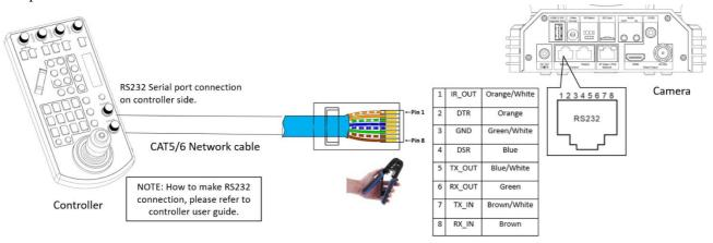
12. How to make RS232 Daisy Chain multiple camera connection with standard RS232 serial port controller as below:
