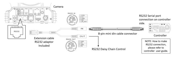
Use extension cables included RJ45 to RS422/232 Phoenix terminal contact adaptor to make RS232 connection for your control device.
