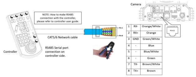
How to make RS485 multiple cameras connection with RS485 standard serial port controller:
