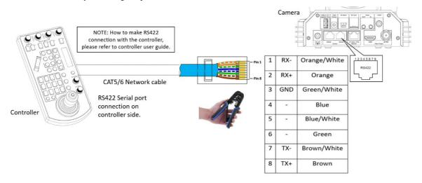
13. How to make RS422 Daisy Chain multiple camera connection with RS422 standard serial port controller:
