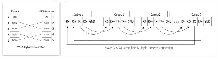
11. Use extension cables RJ45 to RS422 Phoenix connecter adaptor included to make RS422 connection for your control device.
