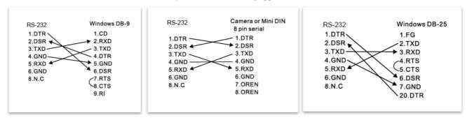
9. Use extension cables included RJ45 to RS232 8 pin Mini Din adaptor to make RS232 connection for your control device.
