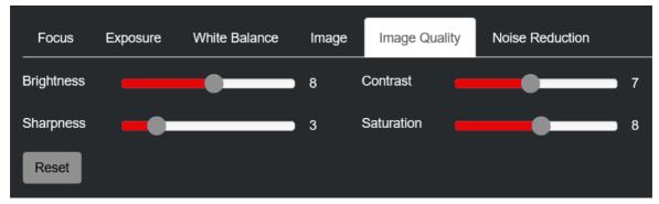
Brightness: You can adjust the values manually for electronic brightness level from 0 to 15
