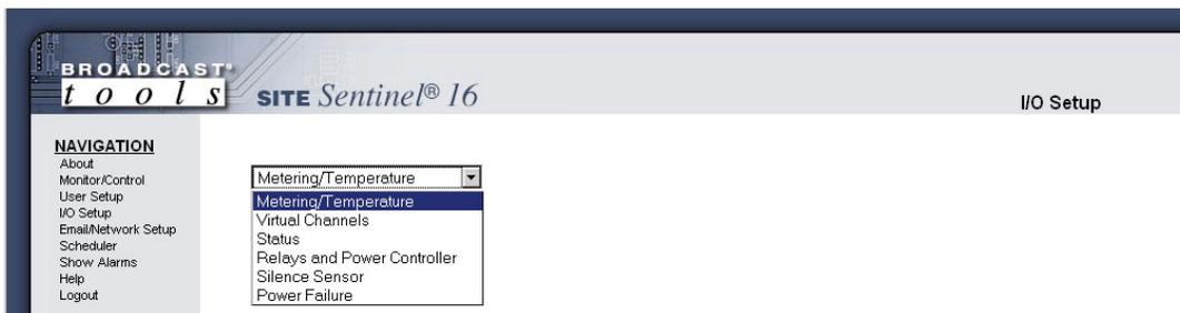
On the I/O Setup screen, choose from the top drop-down box the device to configure.
