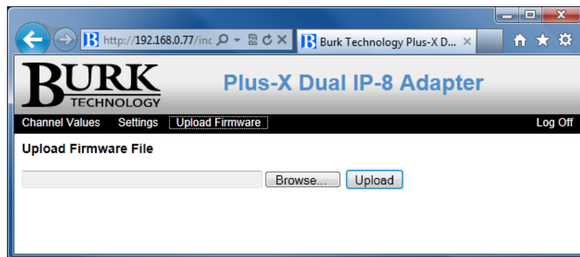
Uploading Firmware to the Plus-X Dual IP-8 Adapter
