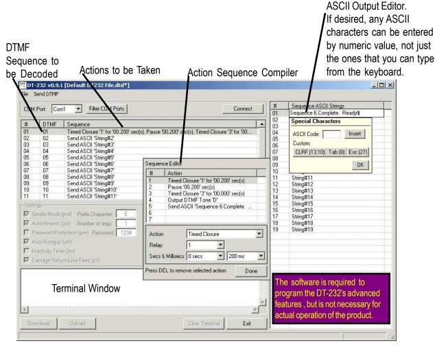
In the DTMF Sequence Mode, actions can include the following functions:
