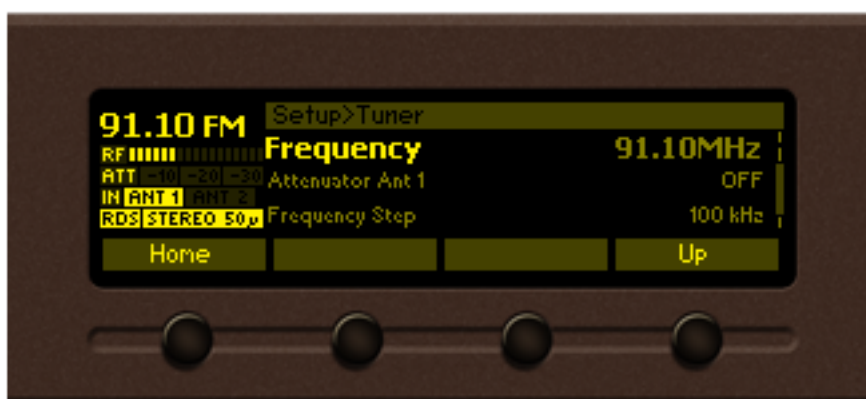
“Frequency” parameter from “Tuner” branch
