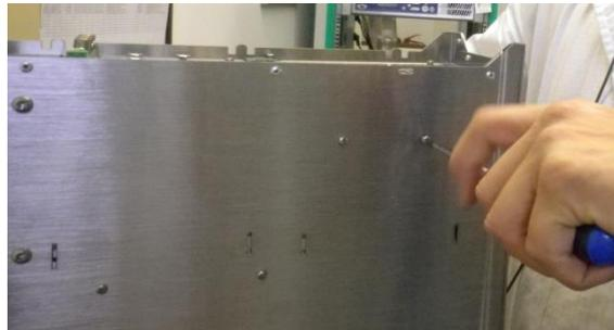
8. Fix the surge suppressor with the mechanical piece **MX01043** and the two M3x6screws (**VIE00180**) from the outside.
