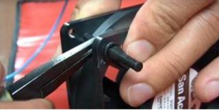
• Insert the legs of the new fan using pliers, making sure of the direction they are facing. Make sure the cable does not get stuck.
