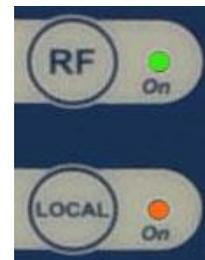
**i** The transmitter is working properly when: the CPU LED blinks, and both the RF LED and the interlock LED are green
