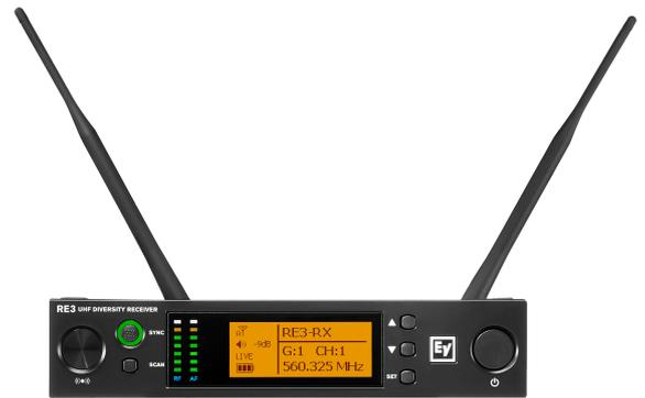
The RE3-RX is a professional rack-mountable, 1/2 space diversity receiver. Designed to function as the control center for an RE3 wireless set, it features frequency scanning and synchronizing, as well as full transmitter control settings which synchronize to a mated transmitter.
