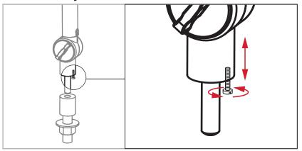
To make fine-tune tension adjustments turn the screw left to decrease tension and turn right to increase tension.
