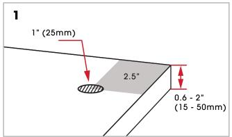
Use a 1" hole cutter and drill out a hole at least 2.5" from the edges of the desk.
