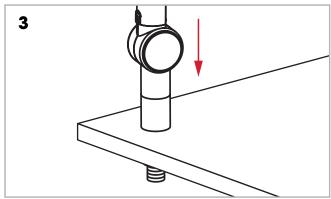
Insert the arm into the hole in the top of the desk insert.
