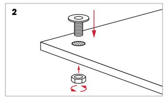
Unscrew the nut from the desk insert and drop it into the hole. Screw the nut onto the desk insert from the underside until it is tight.
