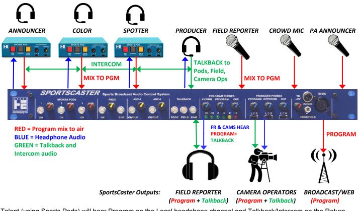
Talent (using Sports Pods) will hear Program on the Local headphone channel and Talkback/Intercom on the Return headphone channel. They can adjust the mix using their Local and Return volume controls. The FR and CAMs will hear a mix of Program and Talkback audio, mixed by the Producer using the SportsCaster FIELD/CAM PHONES volume controls.
