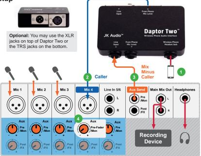
Connect the included CN113 cell phone interface cable between the <Wireless Phone Headset Jack> of Daptor Two and the 3.5 mm TRRS headset jack of your wireless phone or notebook computer.
