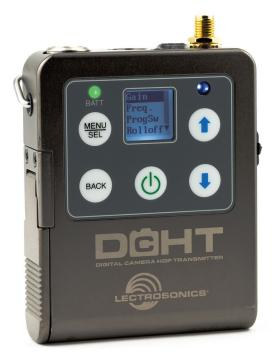
The DCHT, DCHT/E01 transmitter is designed for use in film and television production to provide a wireless link from a bag or cart system to cameras and recorders. The transmitter will accept mic or line level analog signals or AES digital signals from a mixer and transmit the signals to the receiver in a pure digital format. The digital architecture is a fourth generation design with specially developed, high efficiency digital circuitry for extended operating time on two AA batteries.
