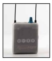
WARNING: Moisture, including talent's sweat, will damage the receiver. Cover the M2Ra in our silicone sleeve (order part # M2RCVR) or other protection to avoid damage.
