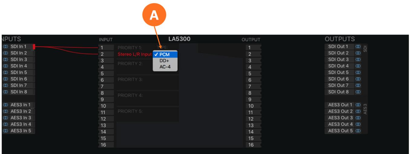
Figure 5 - Selecting the input signal type
