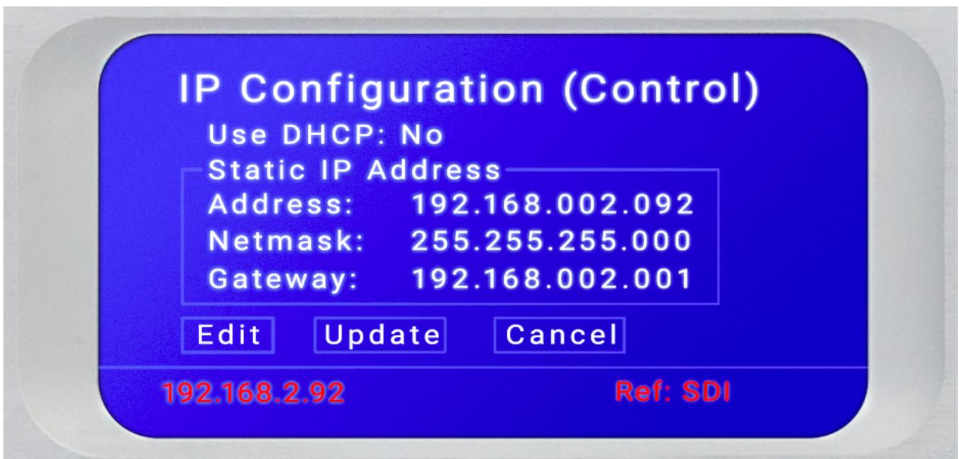
Figure 5 - IP configuration (control) screen
