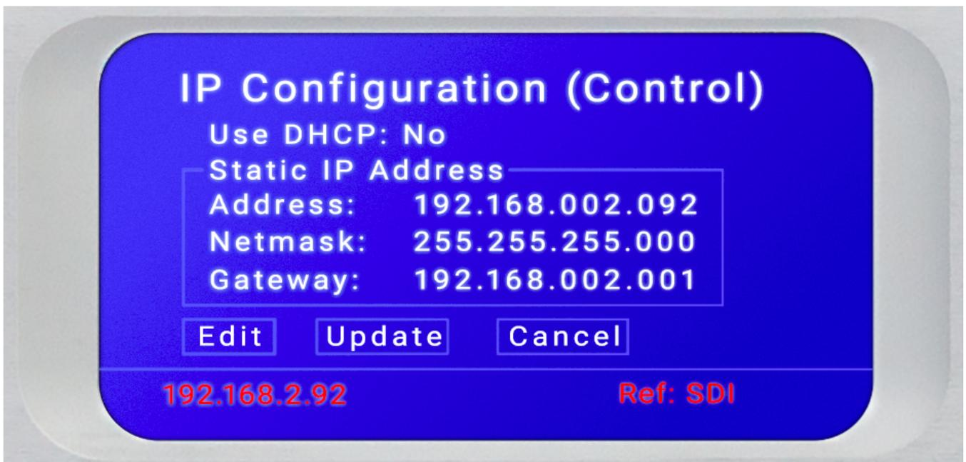
Figure 3 - IP configuration (control) screen
