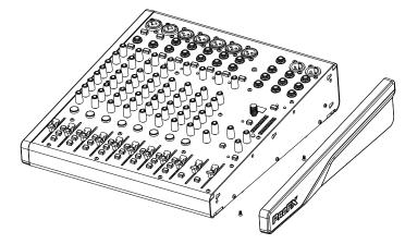
3. Using only the new screws supplied, secure the rack ear brackets to each side of the mixer as shown below. Tighten the screws securely using the Phillips screwdriver. Be sure not to overtighten. As seen in the illustration below, they require eight screws (four on each side).
