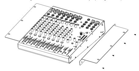
4. Offer up the mixer to the rack and secure it in place with four rack screws (not supplied). Remember to leave enough room at the top to attach the AC power cord and any other connections needed.
