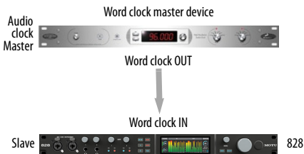
Figure 4-12: Slaving the 828 to word clock. For the 828 clock source, choose Word Clock In .
