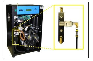
**9.8.3** Use a Voltmeter to measure the DC voltage across each set of "VALVE" terminals.
