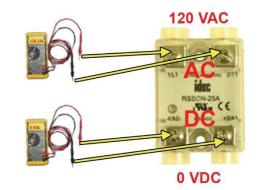
**9.5.6** Use a Voltmeter to measure across the DC terminals. Should measure **0 VDC**.
