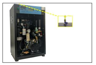
**6.5.7** Install the Plug into the included Precision Bleed Orifice Fitting and then into the dryer Outlet Port.
