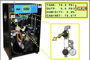
Pressure (OUTP) reading drops below:6.5 PSI for P1500W & P1502W models0.30 PSI for P1500WLP& P1502WLP models
