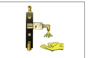
If air flows from this valve continuously the Unloader Valve is defective and should be replaced. See sections 11.2 for part detail and 11.5 for ordering information.
