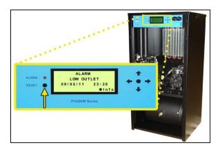
9.16.7 Turn Outlet PressureRegulator knob clockwiseuntil Outlet Pressure(OUTLET) reading raises tothe reading recorded in step9.16.1
