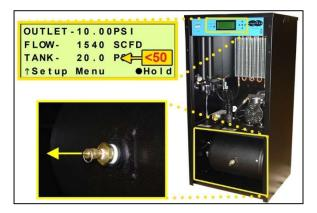
When the Compressor runs for 4:00 minutes (unless adjusted to a different threshold by the user), a Compressor Last Run Time Alarm should appear on the System Screen.
