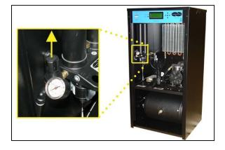
6.5.13.2 Turn the knob until the reading on the Pressure Gauge is 50 PSI (345 KPa).
