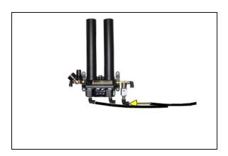
If air flows from this valve continuously the Unloader Valve is defective and should be replaced. See sections 11.4 for part detail and 0 for ordering information.
