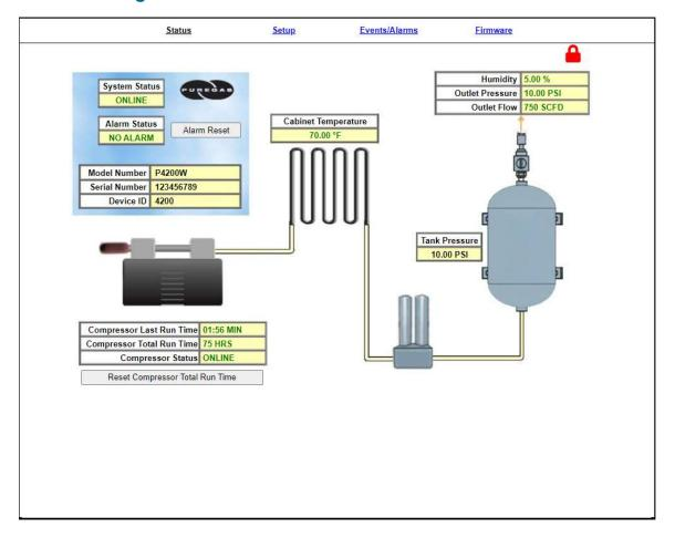
Displays the readings and alarms monitored in the P4200W Series Air Dryer. Provides remote ALARM RESET.
