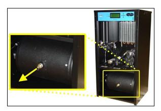
**9.14.4** Unscrew and remove the Humitter from the Combo Block.
