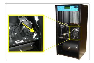
**9.2.3** Use an Amp Meter to measure the Amps of the BLACK wire.
