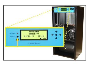
**NOTE:** If the Humitter is disconnected from the Control Board, \*\*% will appear on the Humidity reading and after 5 minutes the unit will Shutdown. This is to allow for troubleshooting.
