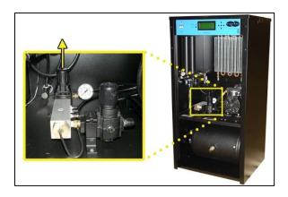
6.5.19.2 Turn knob until the reading on the Pressure Gauge is 20 PSI (138 KPa).
