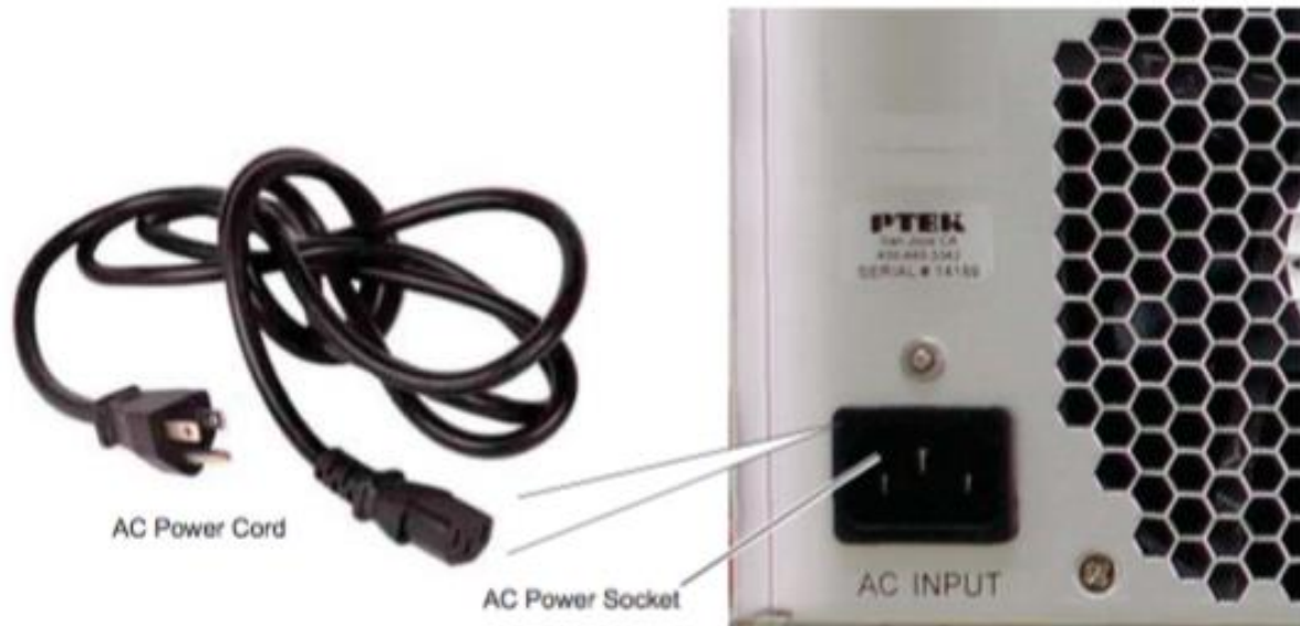
Figure 3-2. Plug the power chord into the transmitter AC Power Socket
