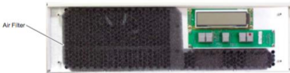
Figure 2-3. Remove the Exposed Air Filter
