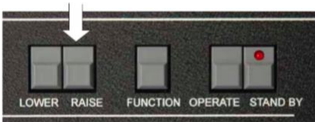
Figure A-2. With the unit in STANDBY mode, press and hold the RAISE Key; then switch the unit from STANDBY to OPERATE
