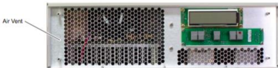
Figure 2-4. Make sure the Air Vent holes are unobstructed
