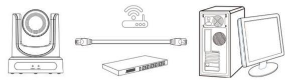
Picture 1.2 Connections to LAN via patch cable to LAN wall jack or LAN Switch
