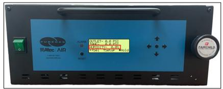
**6.5.16 NOTE**: Press the **RESET** button if the Dryer goes into **SHUTDOWN** mode. If after multiple resets the dryer alarms are still present please proceed to the next steps.
