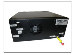
**6.5.6** Remove the plug from the outlet port. And connect your outlet tubing.
