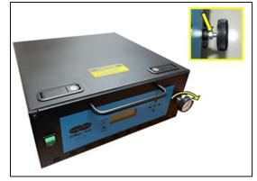
6.5.22.2 Tighten the retaining nut to lock the knob in place.
