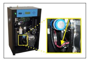
9.2.3 Use an Amp Meter to measure the running amps.
