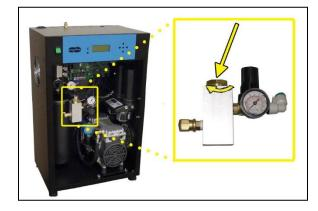
**9.12.7** Press the **RESET Button** to clear the Humidity alarm.
