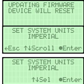
8.7.2.5 Press the Enter (●)Button to confirm the selected choice. This will lock in the new setting.
