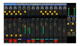
**Quasar Soft -** Unlock your XR or SR's remote capabilities with the optional Quasar Soft Software Upgrade. This customizable remote control solution lets you control your Quasar surface from a browser. You can generate up to eight HTML-5 pages and configure them to display any of the 64 input channels, plus a small monitor section, or even the entire master section of the console.
