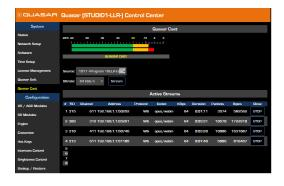
**Quasar Cast -** Included as part of the Quasar Soft license, Quasar Cast is a remote monitoring solution that lets you listen to any Livewire stream in the network through the same web browser. Quasar Cast generates a compressed OPUS stream from a source in the Livewire® network and can serve up to eight clients (including Quasar Soft instances). With Quasar Cast, you can listen to what is happening in the studio, and on the air, while you operate the console remotely using Quasar Soft.
