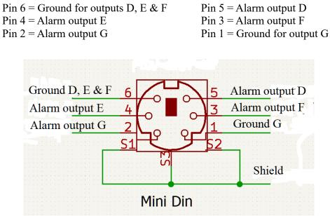
Figure 3: 6 Pin Mini DIN connector
