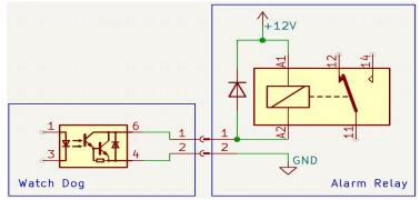
Figure 4: Alarm Relay Driver Example
