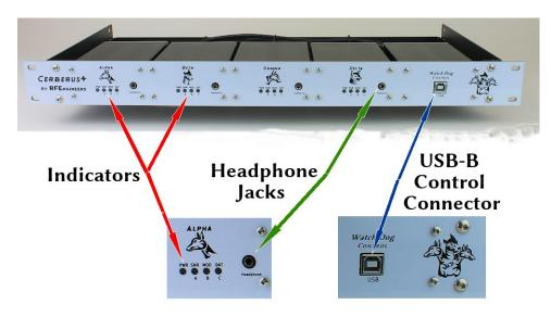
Figure 1: Front Panel Features
