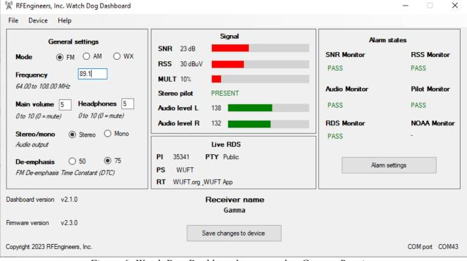
Figure 6: Watch Dog Dashboard connected to Gamma Receiver
