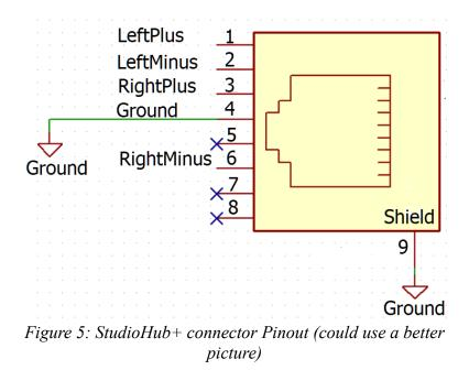
The WDC receiver's rear panel RJ45 connector is *balanced* (differential) audio. It should **NOT** be connected to an *unbalanced* load without proper matching devices. There are many sources of such matching devices and StudioHub+ adapters available from your favorite supplier.
