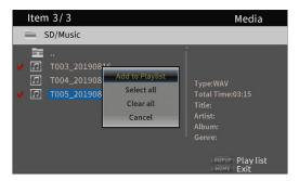
• In addition, check marks can be added to all files in the folder by selecting "**Select all**" in the pop-up and pressing the **ENTER** button in step 3.
