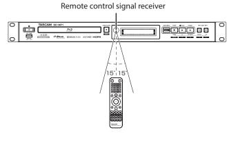
Remote control operation range From any angle within 15° of front: 5 m
