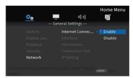
Use the > cursor or **ENTER** button to move to the function setting. Use the  $\checkmark/\land$  cursor buttons to select "**Enable**" or "**Disable**" and press the **ENTER** button to confirm. To exit a folder or subfolder, press the  $\leq$  cursor button
