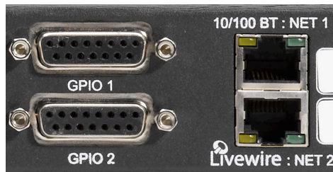
Fig. 1-5: GPIO and Livewire network connections
