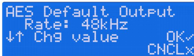
Figure 7 - AES output rate screen
