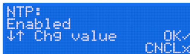
Figure 3 - NTP enable screen
