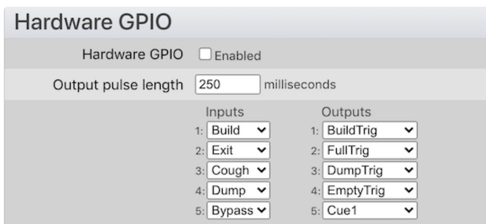
Figure 3- Hardware GPIO
