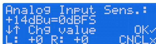
Figure 5 - Input sensitivity screen
