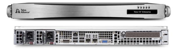
VX Enterprise 1RU rack-mount device is the heart of the system. It provides all the call control and audio processing needed for the system, and supports up to 120 active calls on-air simultaneously. Its two Gigabit Ethernet ports provide a cost-effective interface to both telephone lines and studio audio via proven Livewire AoIP. VX Enterprise is Web-based, so remote control and configuration are a snap — engineers can work with it from any place they can get online.
