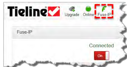
Fuse-IP enabled & tunnel created
