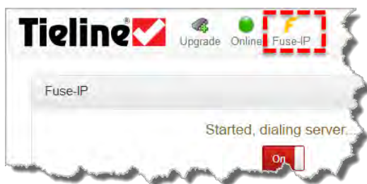
Fuse-IP Enabled & no tunnel created
