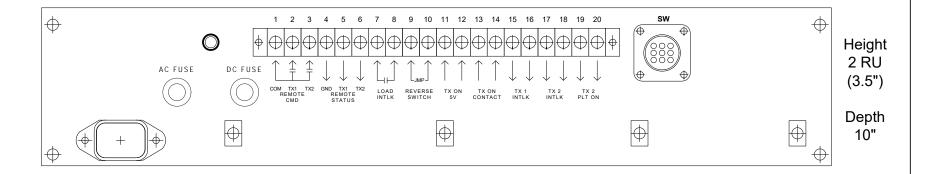
For 1 coax switch, 2 transmitters, 1 antenna, and dummy load. Safe switching from a single momentary local or remote command.
