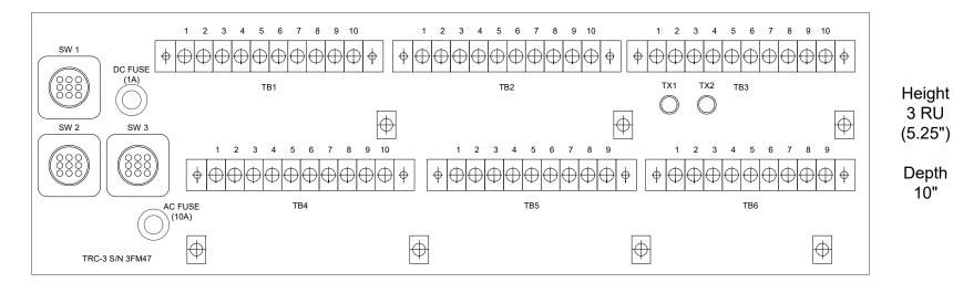
For 3 coax switches and combiner, IBOC or analog. Safe switching from a single momentary local or remote command. Logic for a third transmitter is programmed.
