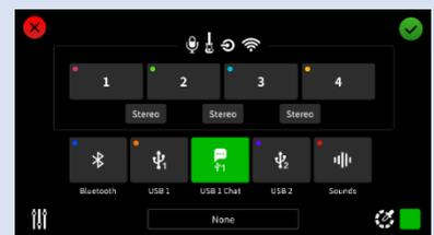
8. Optional: configure the output routing for USB 1 Chat to send a custom audio mix to the CallMe-T codec (i.e. SIP destination), instead of the default mix-minus, by tapping Settings
