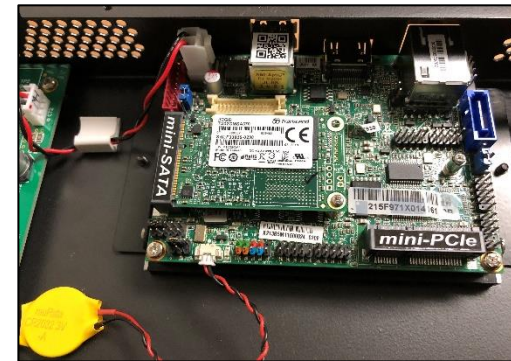
Figure 5-2 LXE Surface Host mounted in Mix Engine
