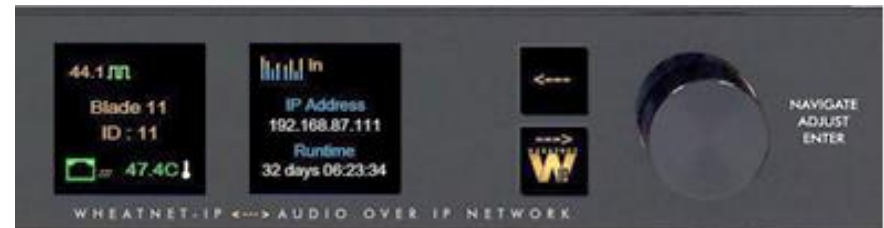
Figure 3-3 Mix Engine Front Controls, System Info Displays
