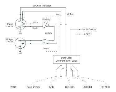
The block diagram above shows the functional structure of the hush<sup>+</sup> device. In contrast to hush, hush<sup>+</sup> offers you control options for your microphone signal. hush<sup>+</sup> comes with a high-quality microphone preamp. It offers you various options optimizing and controlling your mic signal, e.g. a mute function. See page 31.
